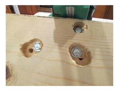
Countersunk holes on bottom of base
